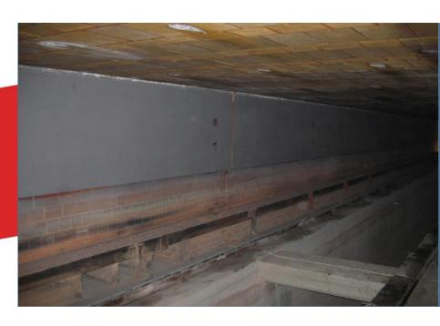
Insulcoat 1260-RFL, an energy-saving reflective coating Energy-saving in thermal process plant, including tunnel and bogie hearth kilns in the ceramics industry, is a topic which has received a great deal of attention in recent years.
