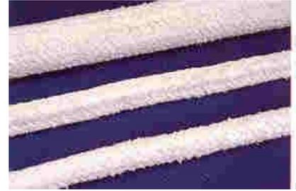
**Keramab® braided packing** is reinforced with glass (650°C) or metal wire (1050°C) and contains approximately 20% organic carrier fibre to facilitate the carding process. The carrier fibre burns out at a low temperature, but this has no effect on the properties of the ceramic fibre.
